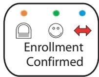
**After completion of Enrollment:** The Blue LED will stay on, but the solid Orange LED will disappear. **At this time, Set the Enrollment switch to normal and disconnect from USB port. (You can now use your BioStik™)**
